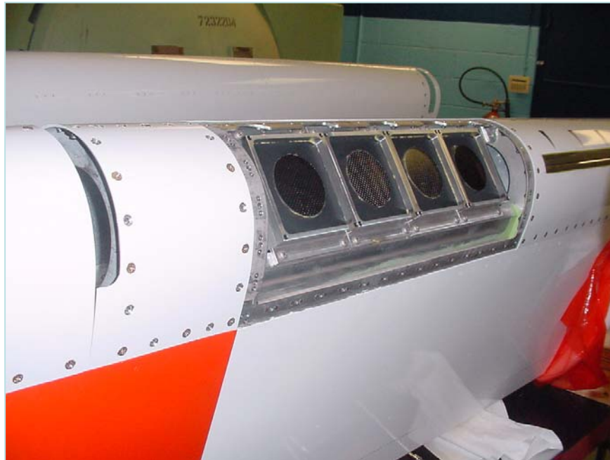
Figure 27: ATEAM-15 Actuators Installed in the XV-15 Flap.
