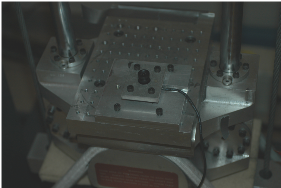
Figure 12. Camera fixture mounted to MTS shock table.
