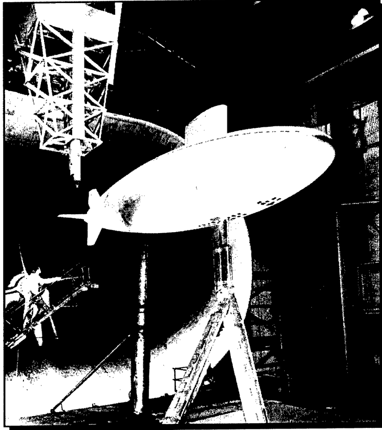
Figure 6. Albacore being tested in a wind tunnel [7]
