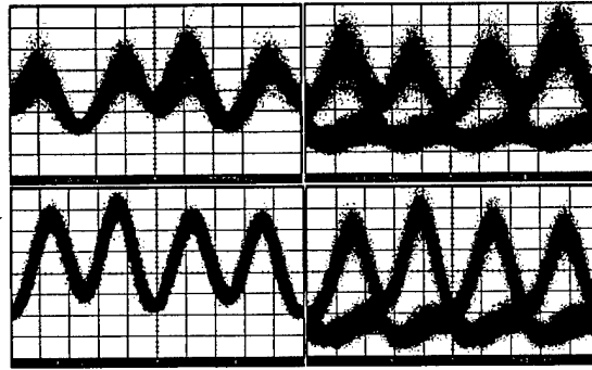
Figure 8. Top left (a): Trace of 40Gb/s pulse train w/o use of SOA. Top right (b): Corresponding eye-diagram. Bottom left (c): Trace of 40Gb/s pulse train w/ use of SOA. Bottom right (d): Corresponding eye-diagram.
