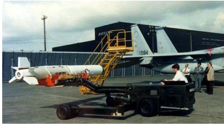
Figure 6. USAF Air Launched ASAT ASM-135A. Photo taken at Edwards AFB CA Flight Test Center.
