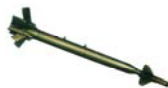
Figure 7 Schematic of a GBU-28. It is an un-powered, hard target laser guided weapon.
