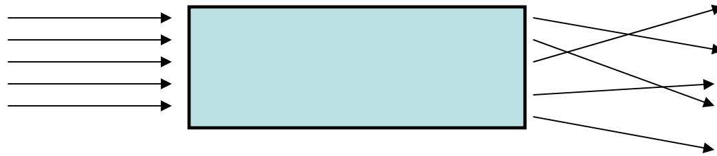
Laser amplifier with inevitable phase inhomogeneities
