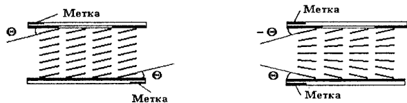
Fig.1. Distribution of the director of molecules NLC in a microlens at a zero potential on control electrodes: a) identical pretilt of molecules; б) opposite pretilt.
