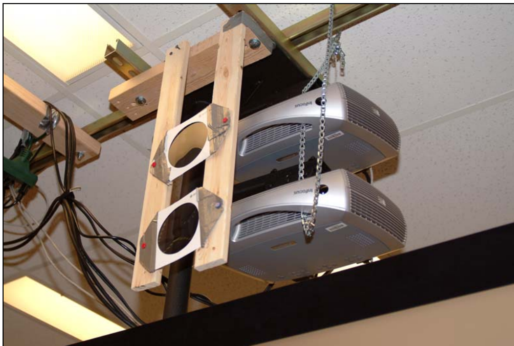
Figure 3. Dual DLP projectors with polarizing filters.
