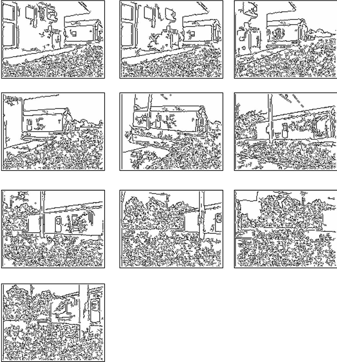
Figure 12. Edges in VS1 as determined by the Canny edge detector component of the NVLD procedure.
