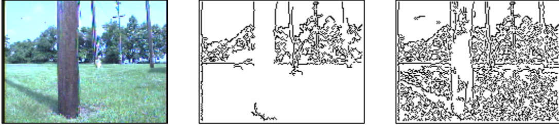
Figure 3. Results of Canny edge detection: original image (left); edges with t(\text{high}) = 0.95 (center); edges with t(\text{high}) = 0.5 .
