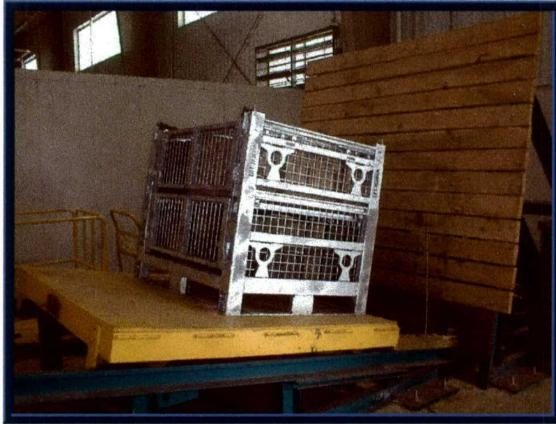
Photo 19. Incline-Impact Testing of the ISTF Unit #2.
