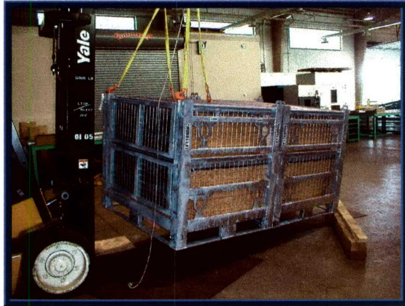
Photo 24. Cornerwise Rotational Drop Test of the Interconnected ISTF-2 Units.
