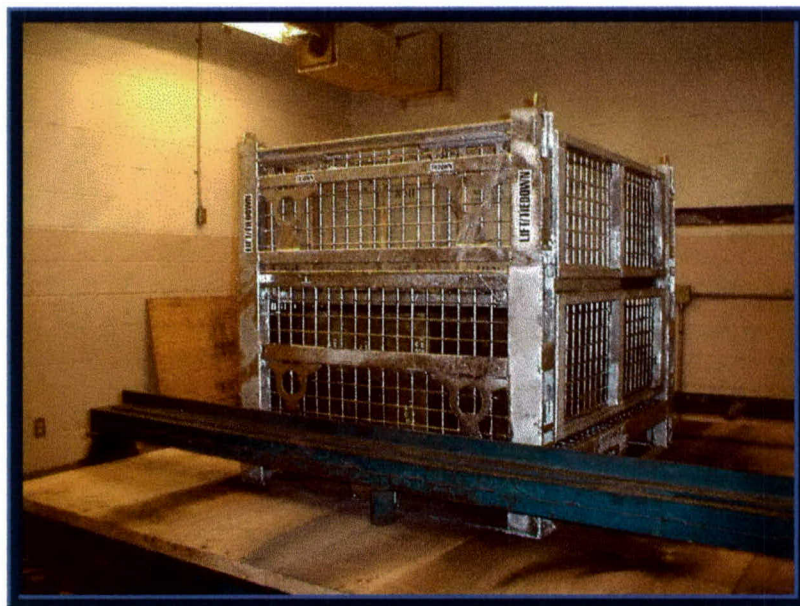
Photo 17. ISTF-2 Unit #2 During the Repetitive Shock Testing.
