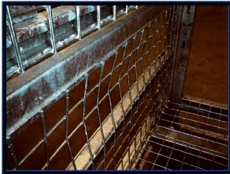
Photo 9. Bent Wire Mesh of the ISTF-2 Unit #1.
