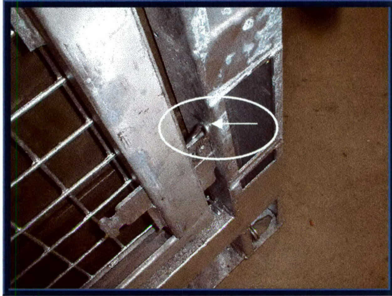
Photo 10. Bent Locking Clip on ISTF-2 Unit #1 Slider.
