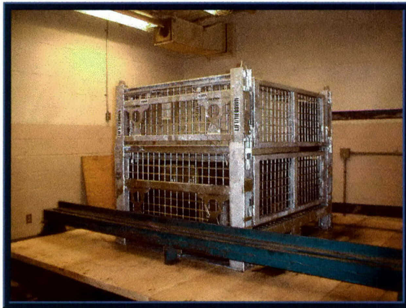
Photo 2. Example of the Repetitive Shock Test. (ISTF-2)
