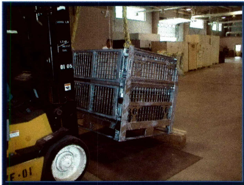
Photo 18. Edgewise Rotational Drop Test on the ISTF-2 Unit #2.
