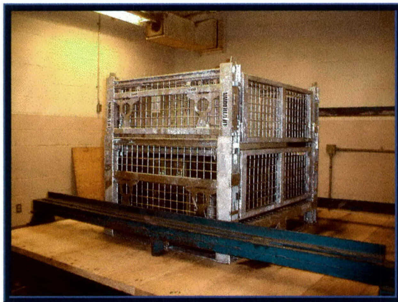
Photo 6. ISTF-2 Unit #1 During Repetitive Shock Testing.
