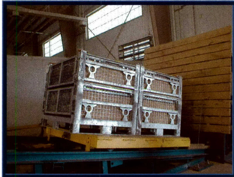
Photo 28. Incline-Impact Testing of the Interconnected ISTF-2 Units
