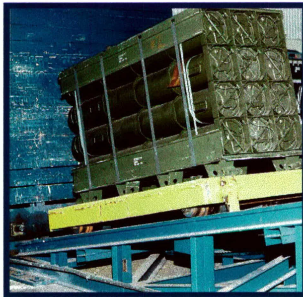
Photo 4. Example of the Incline-Impact Test. (2.75-Inch, Hydra 70, PA151 Rocket Pallet on incline-impact tester.)
