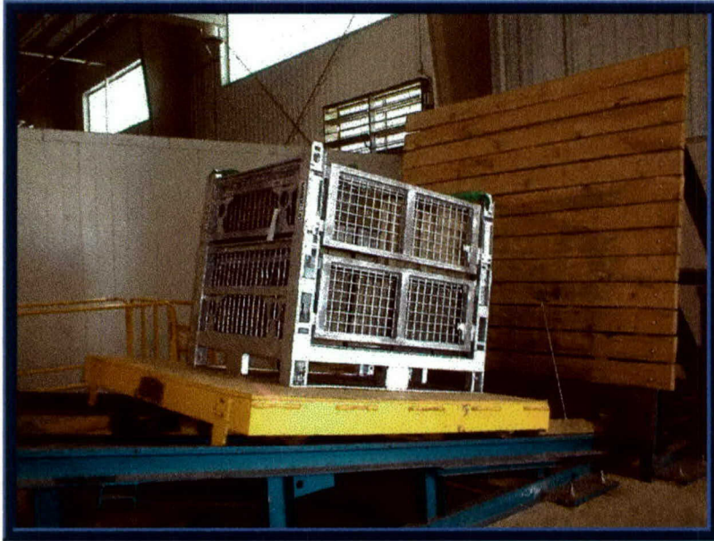
Photo 8. Incline-Impact Testing of the ISTF-2 Unit #1.
