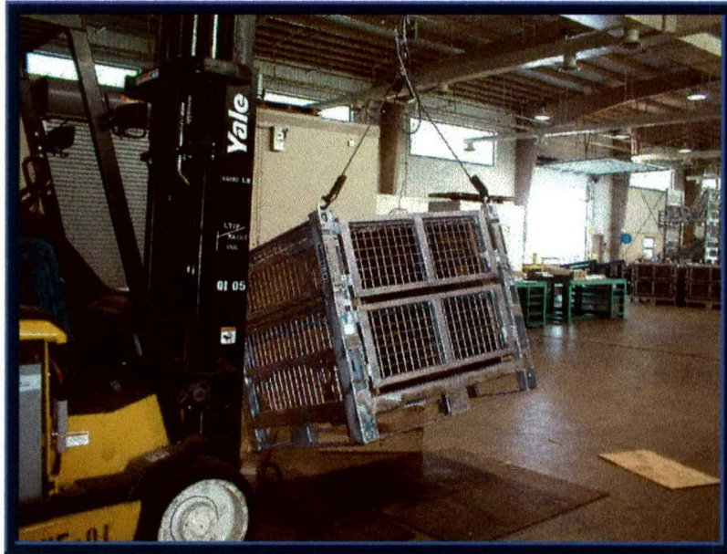
Photo 23. Cornerwise Rotational Drop Test on the ISTF-2 Unit.
