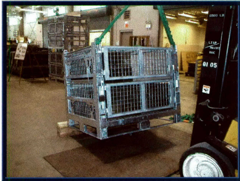
Photo 7. Edgewise Rotational Drop Test on the ISTF-2 Unit #1.
