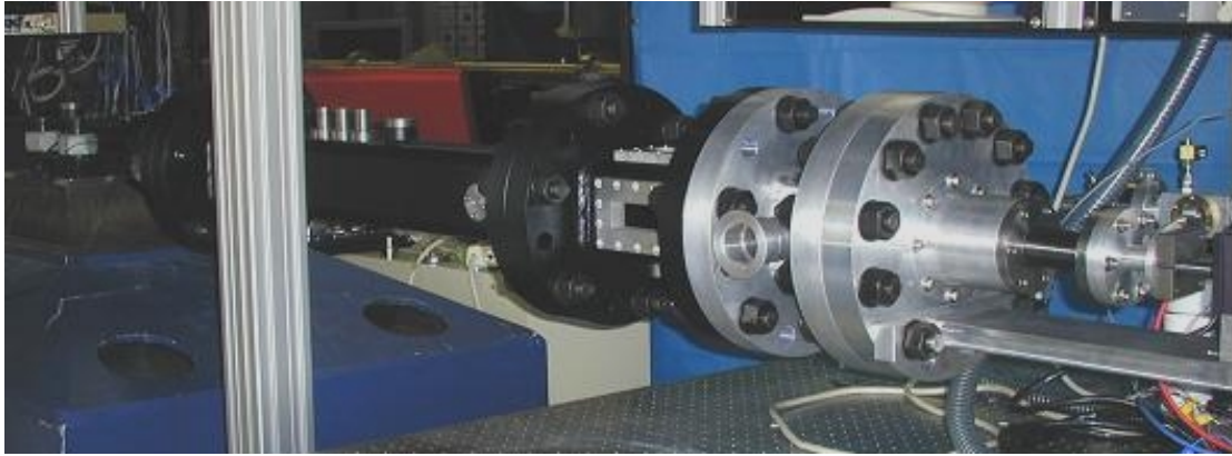
Figure 8. Detail of aerosol shock tube end section. The black epoxy coated pieces are the transition and viewing section; the aluminum section with black bolts houses the four flush-mounted poppet valves in the endwall.
