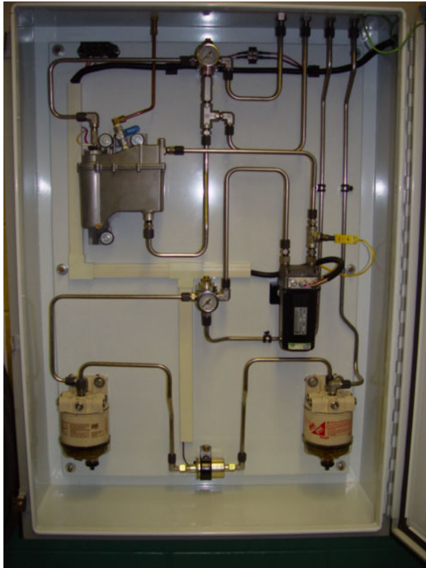
Figure 1.2.2: Fuel delivery system.
