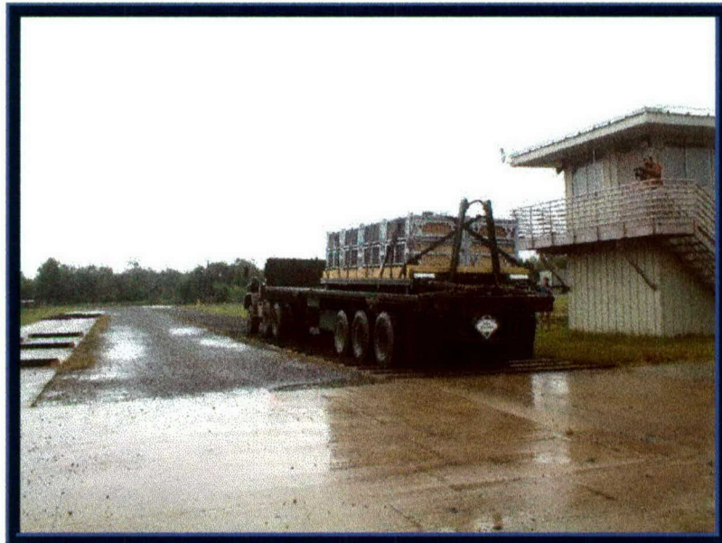
Photo 15. Washboard Course Testing of the ISTF-2s on a Summa CROP
