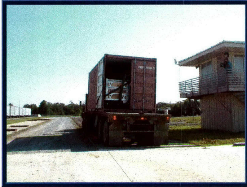
Photo 10. Washboard Course Testing of the ISTF-2s on a Hyundai CROP
