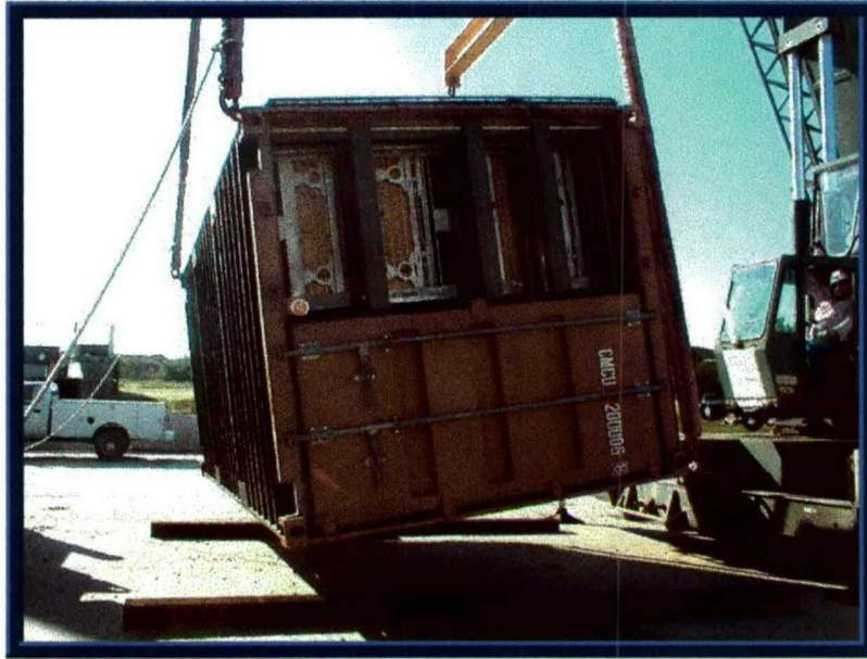
Photo 6. Tilt Testing of ISTF-2s in an End-opening Container
