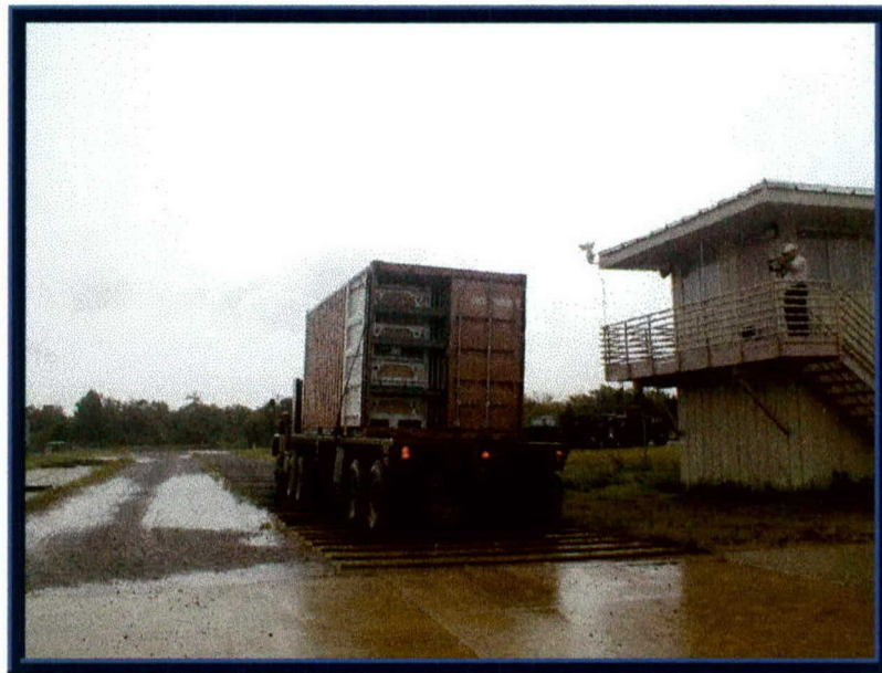
Photo 5. Washboard Course Testing of the ISTF-2s in an End-Opening Container
