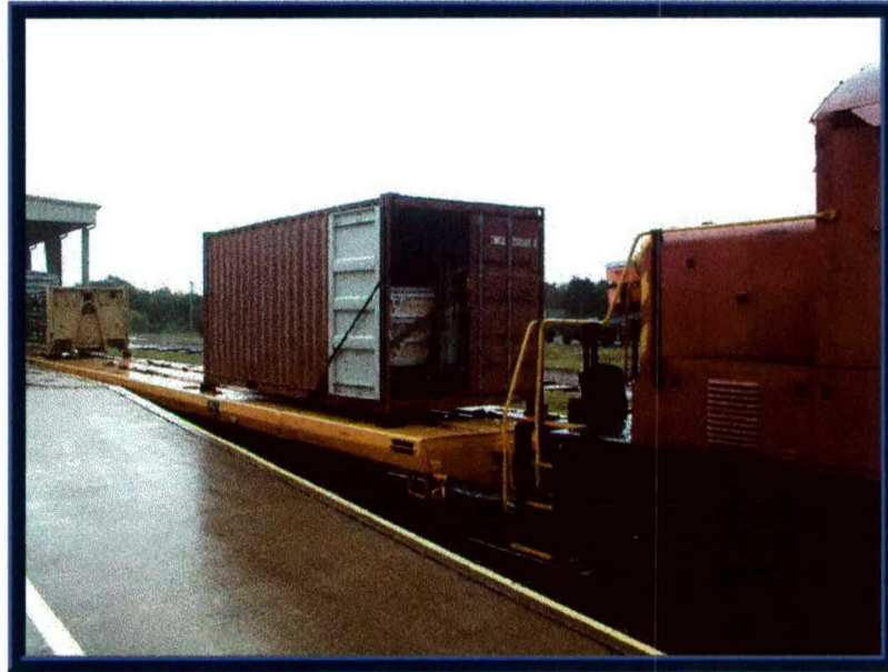
Photo 8. Rail Impact Testing of the ISTF-2s on a Hyundai CROP (Prior to Testing)
