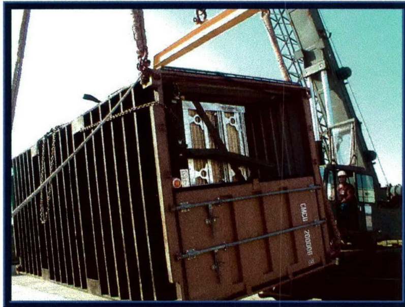
Photo 11. Tilt Testing of ISTF-2s on a Hyundai CROP
