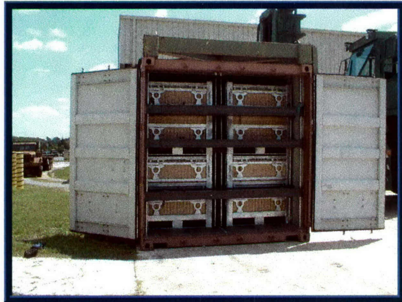
Photo 1. ISTF-2s in an End-opening Intermodal Container
