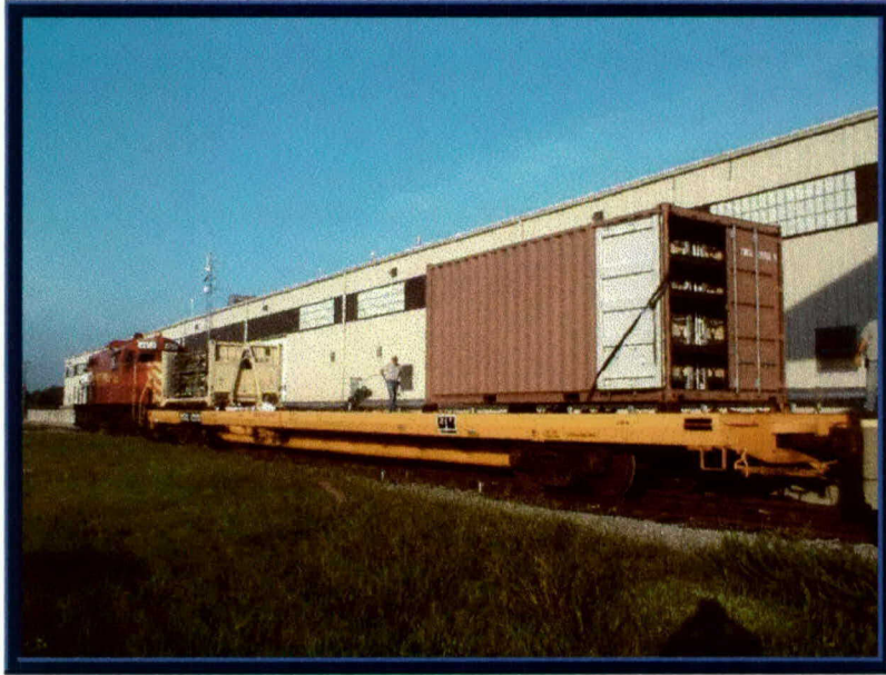
Photo 2. Rail Impact Testing of the ISTF-2s in an End-opening Intermodal Container (Prior to Testing)
