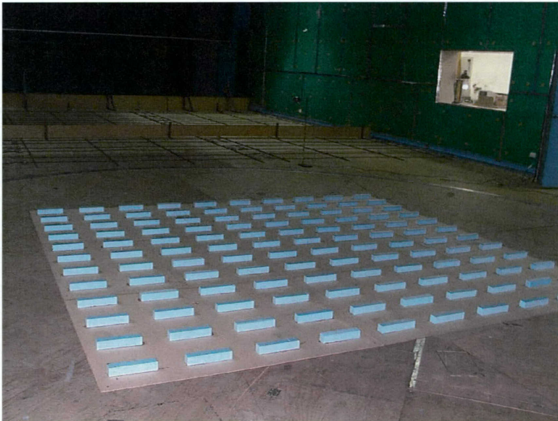
Figure 2.2: A photo of the Monash University wind tunnel facility, with the model of the MUST array, flow conditioning trip boards and a window to the control room all in view.
