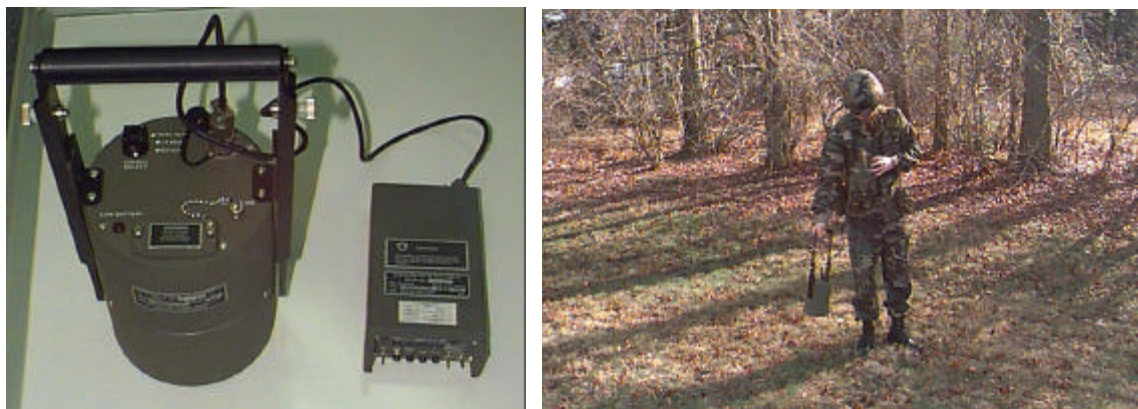
Figure 7-F: The X-Ray probe and the control unit is shown on the left. The proper use of the probe is shown on the right.
