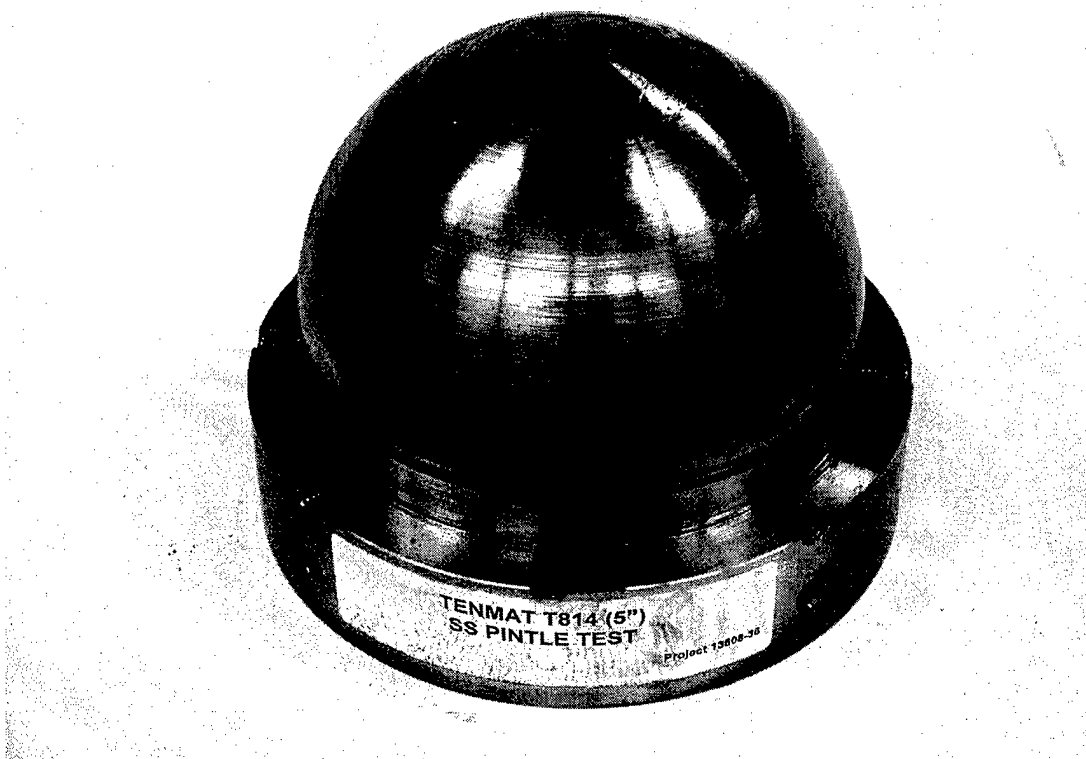
Figure D1. Overview of 5" Tenmat T814 pintle. Due to the thickness of the bushing-retaining ring, the first row of pintle anchoring holes had to be machined away.
