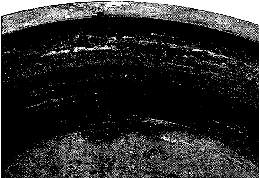
Figure B9. Close-up view above image on loaded side. Note accumulation of wear debris above darker contact area.
