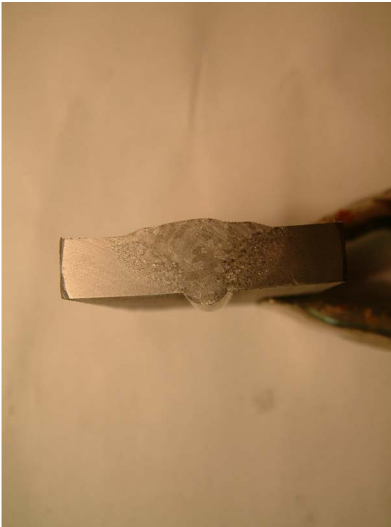
Fig.6. Symmetrical butt weld produced by torch with magnetic device.
