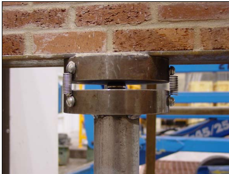
Figure 2-7. Pin connection for steel support column.
