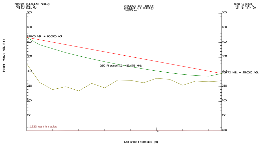
Figure B18. Point-to-point radio communications study for Master Repeater to Lift Station #18.
