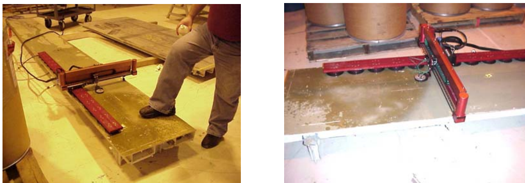
Figure 14: MAUS second layer ultrasonic procedure preliminary validation at Boeing-Wichita
