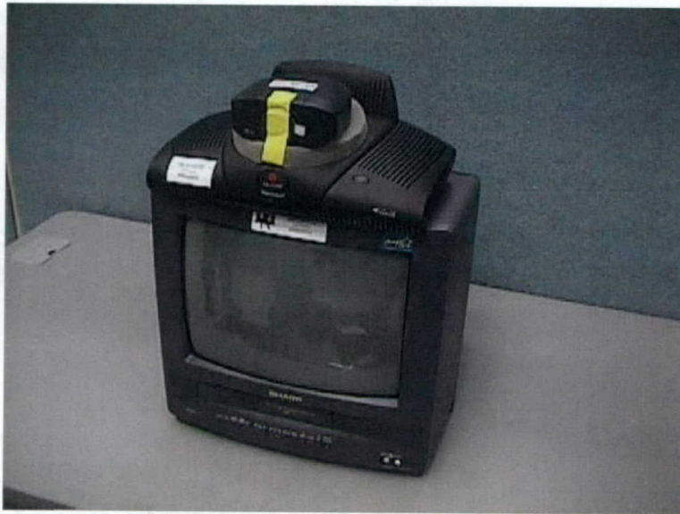
Figure 8. Polycom ViewStation positioned on TV
