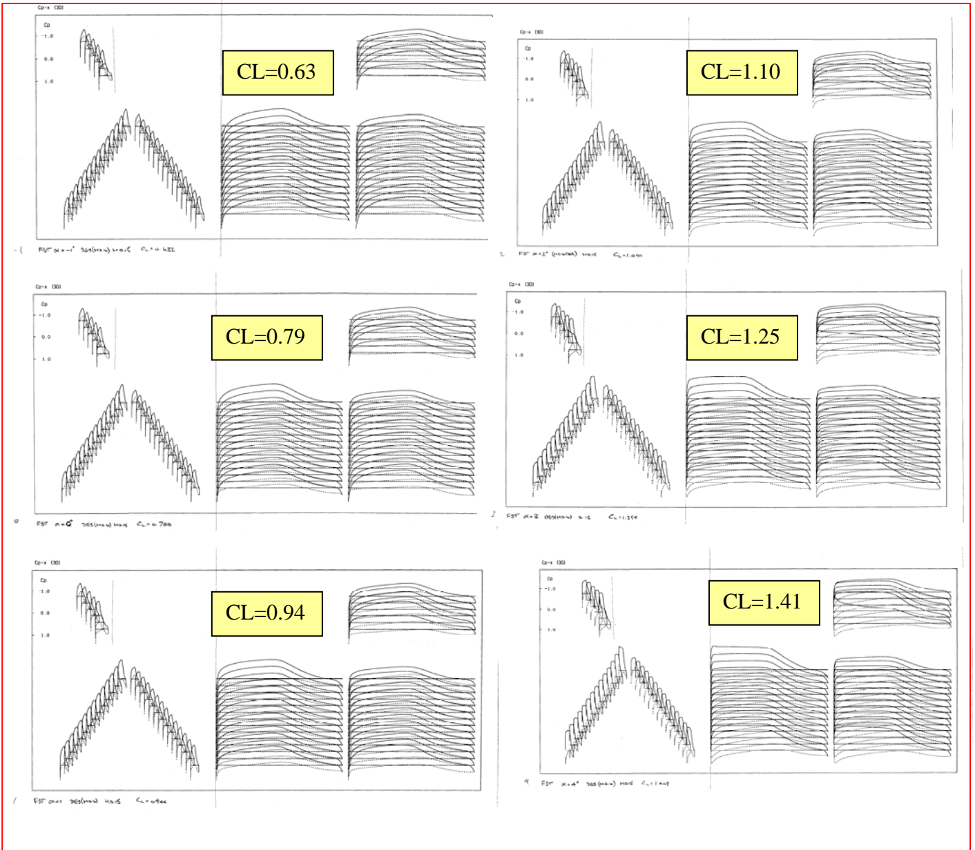
FIG. 7.2.3 CONFIG. FT1, DESIGNED, Cp DISTRIBUTIONS THROUGH AoA RANGE, Mach 0.15
