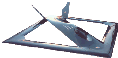
FIG. 1.2 POSSIBLE INTAKE LAYOUTS ON JOINED WING AIRCRAFT
