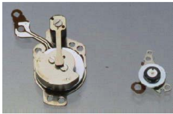
Figure 23 Micro-ultrasonic motors utilized for silent alarm (8 mm diameter, left-side) and date change (4 mm diameter, right-side) mechanisms in a wristwatch (SEIKO, Japan). 19
