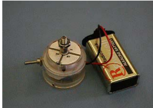
Figure 10. Battery-operated ultrasonic motor (hula-hoop type) with a piezoelectric transformer (ring-shape) integrated in a drive circuit.
