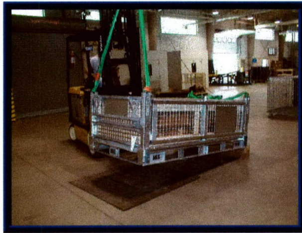
Photo 3. Example of Edgewise Rotational Drop Test (Plastic XYTEC 4845 Pallet Box)
