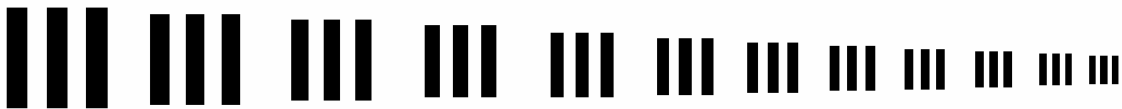
Figure 11. The Modified USAF 1951 Test Pattern Showing Vertical Bar Patterns Arranged Across a Line [Adapted from Edmund Optics]
