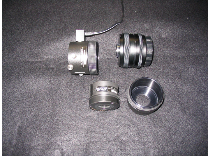
Figure 38. Basic Components of Astroscope 9350 (Clockwise from top left, Power unit and C-mount adapter, Objective lens, C-mount device for objective lens, Central Intensifier Unit)
