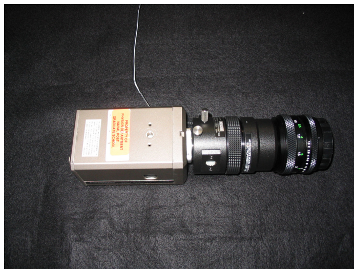
Figure 39. Complete Assembly of Astroscope 9350 with Camera
