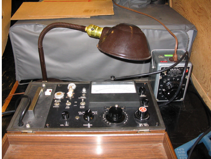
Figure 16. The 2020 Photometer and Variac Driver (Right)
