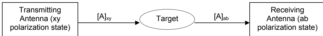
Figure III-4 Polarization States of Transmitted and Backscattered Waves
