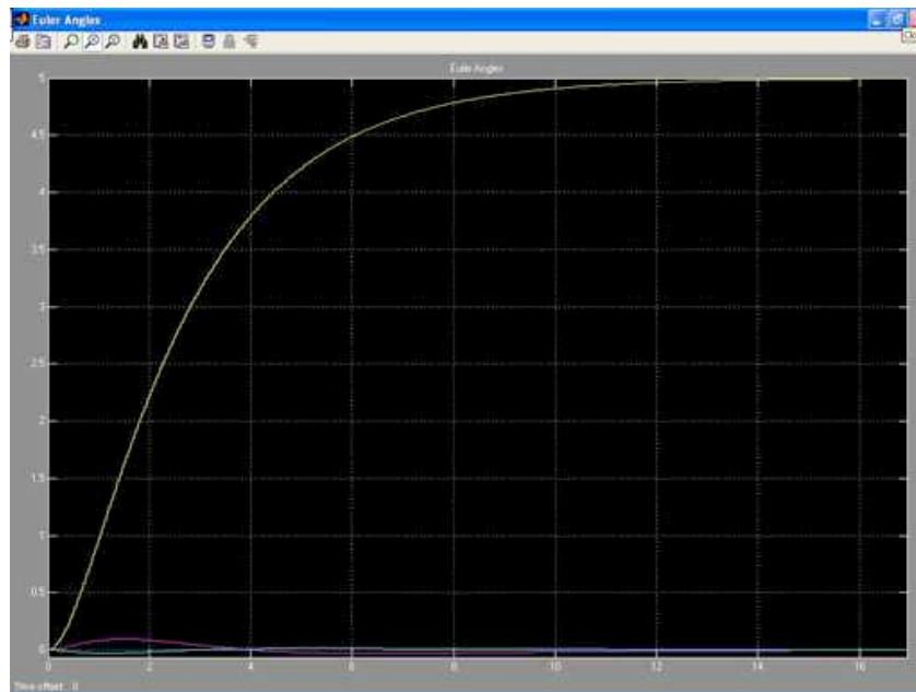
Figure 38. Euler angles, 5 degree slew about +X, ideal Critically damped, rise time ( T_r ) can be seen to be 5.25 sec, settling time T_s = 10 sec.
