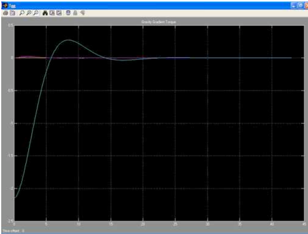
Figure 51. Gravity torque, 2mm CG offset, worst case
