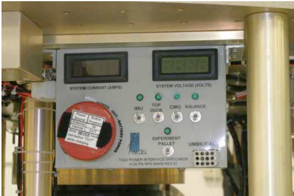
Figure 14. Power switch box
