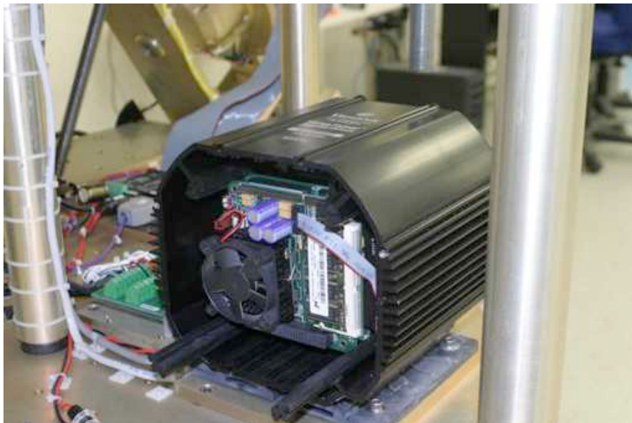
Figure 24. Industrial Embedded Computer (IEC)
