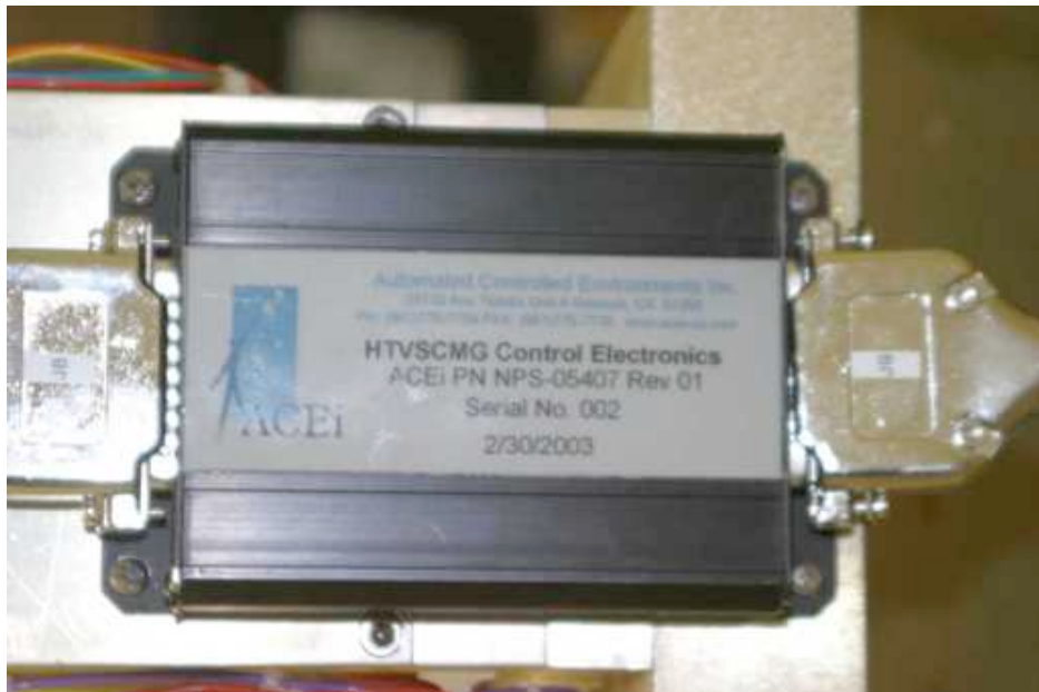
Figure 9. CMG Rotor speed controller
