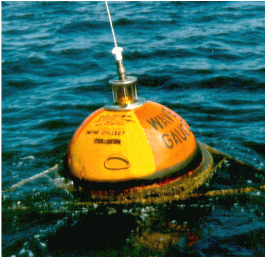
Figure 7. Datawell Waverider Buoy. This particular buoy is fitted with an anti-spin triangular frame to reduce the risk of damage from collisions. (From: www.cdip.ucsd.edu )
