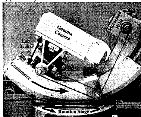
Figure 3: The current dedicated emission mammotomography system. The lab jack(s) provide for changes in the radius-of-rotation (ROR); the goniometer allows polar ( \phi ) camera tilt; and the rotation stage provides for azimuthal variations ( \theta ).
