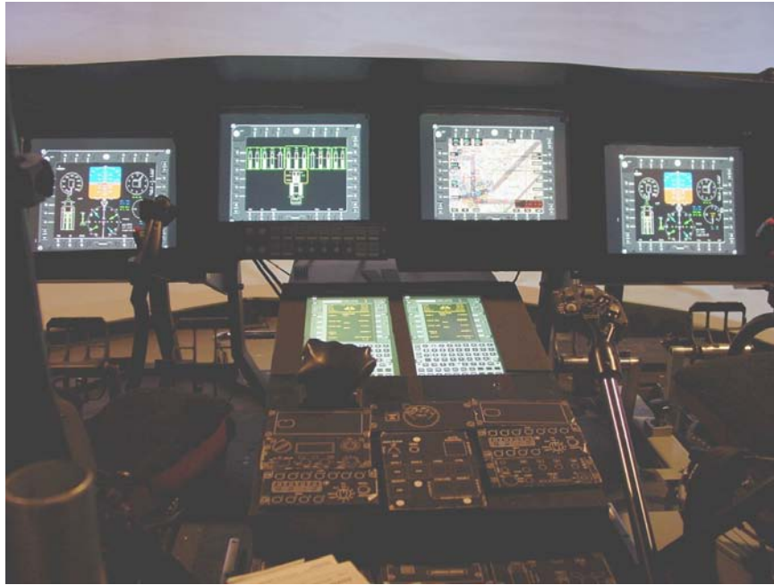
Figure 5. UH-60M BHIVE crew station used for EUD2. (Note that the MFDs and FMS are replicated with touch screens versus actual hardware; courtesy of AMRDEC and Science Applications International Corporation.)
