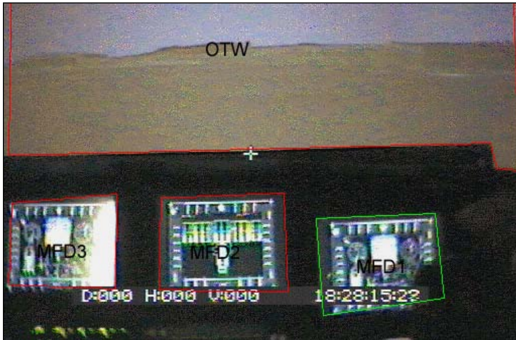
Figure 7. Eye tracker FOV and data capture viewing planes. (OTW = out the window.)
