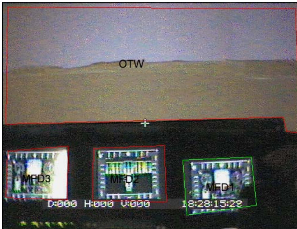
Figure 16. FOV with the eye tracker camera.
