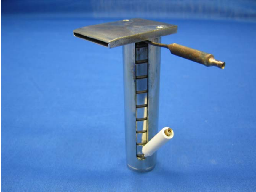
Figure 8. Photograph of an assembled Cs injector.
