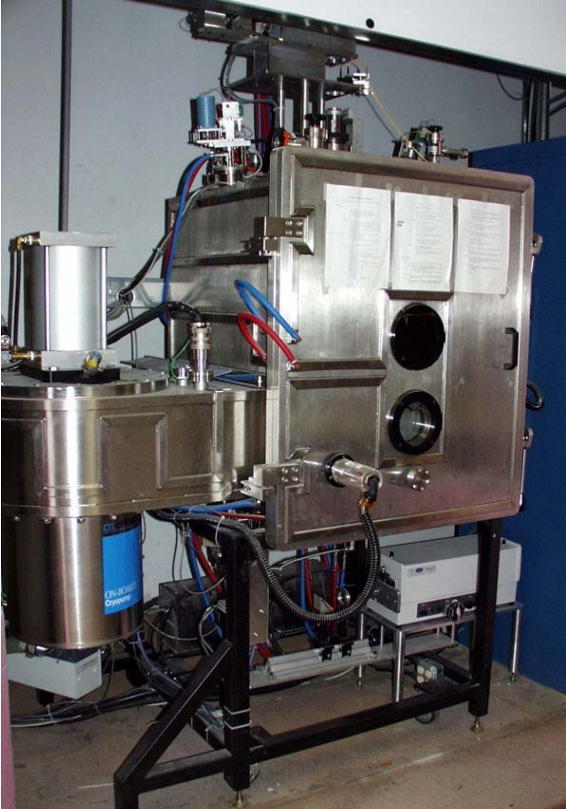
Figure 4: Represents the vacuum chamber purchased and modified for Ion Beam Deposition of Optical Coatings
