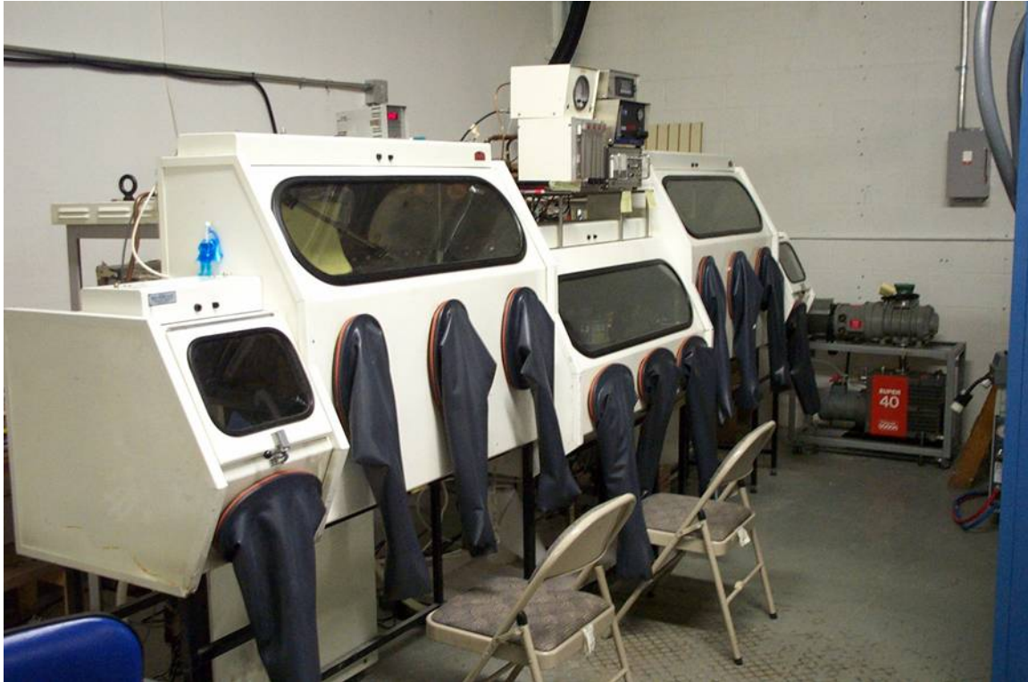
Fig.6 A photograph of the new glove box for handling Cs and loading it into cartridges in an Ar atmosphere.
