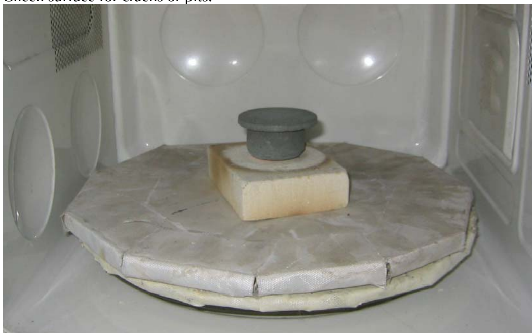
Figure 16 Silicon carbide crucible set-up in microwave oven.
