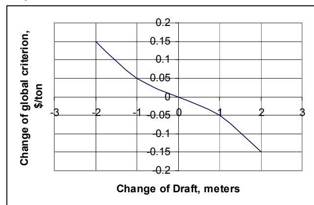
Figure 8: Economical criterion versus maximum draft. Relative cost of draft is 0.04 [$/t / m] or 95,000 $/meter.
