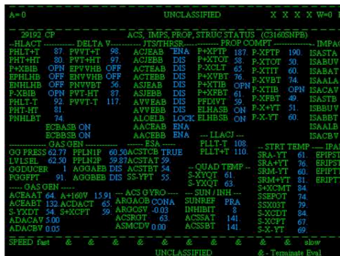
Figure 1: Example of a satellite operator screen employing ineffective use of color and inexplicit mnemonics
