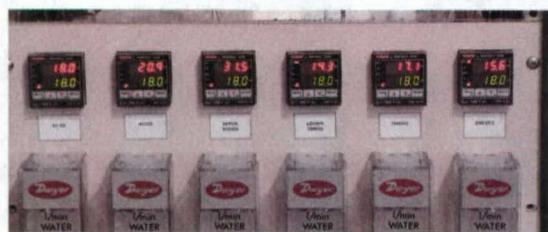
Figure 4. Proportional control units for the in-line water heaters
