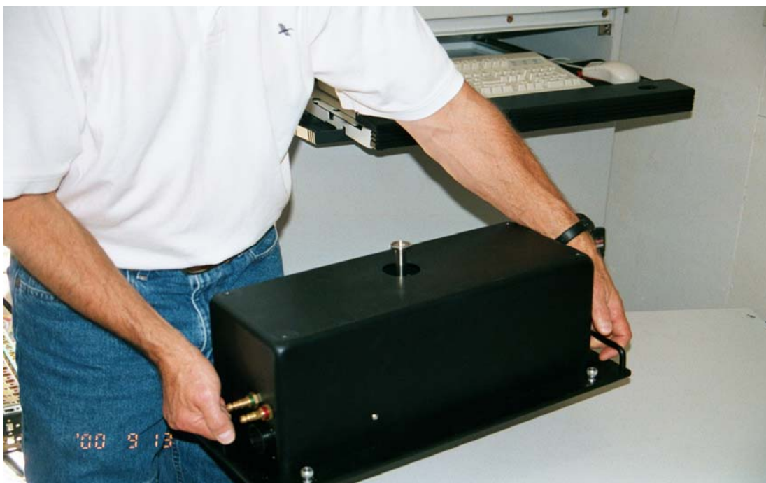
Figure 3. XCEM sampling cassette.
