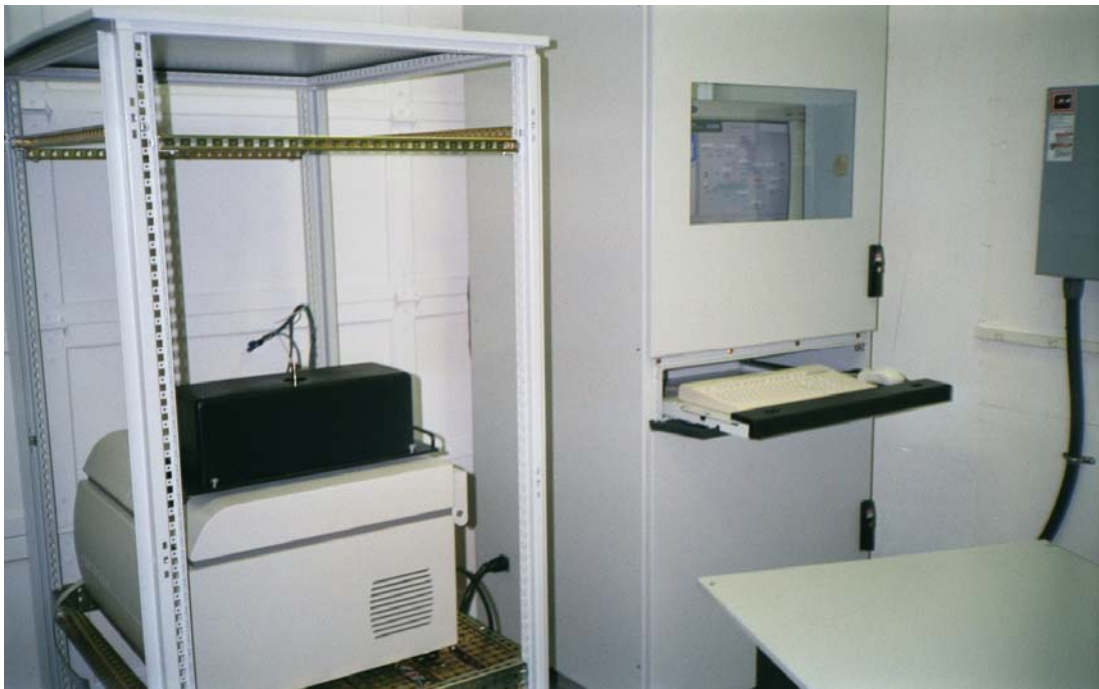
Figure 2. XCEM analysis system, computer control, and sampling cassette.
