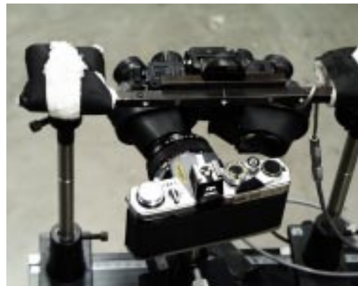
Figure 5. Geometric arrangement to photograph both the left central and outboard oculars of a PNVG II.
