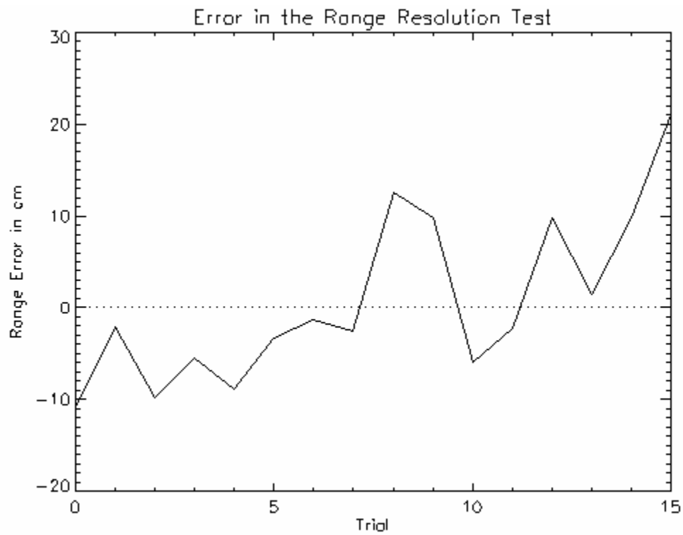
Figure 32-b: Plot of range resolution error
