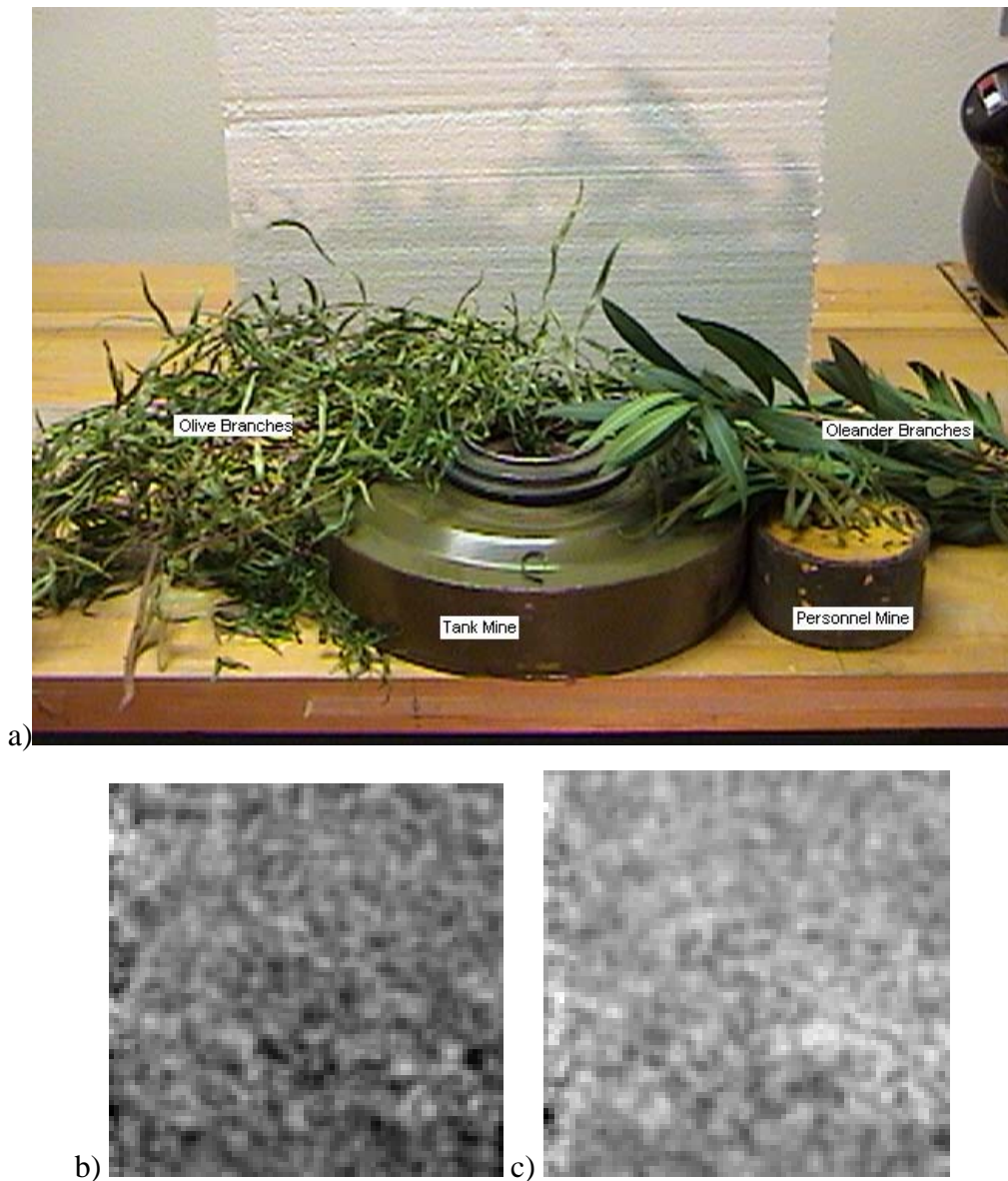
Figure 48: a) Photograph, and range images of the target under b) Range reconstruction for laser only illumination and c) Range reconstruction for laser and ambient illuminations (Range images are scaled to show the detail).
