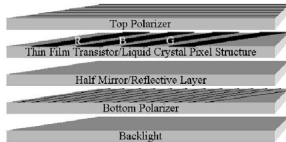
Figure 1. Transflective display structure
