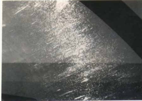
Figure 2.5: Example of crazing.
