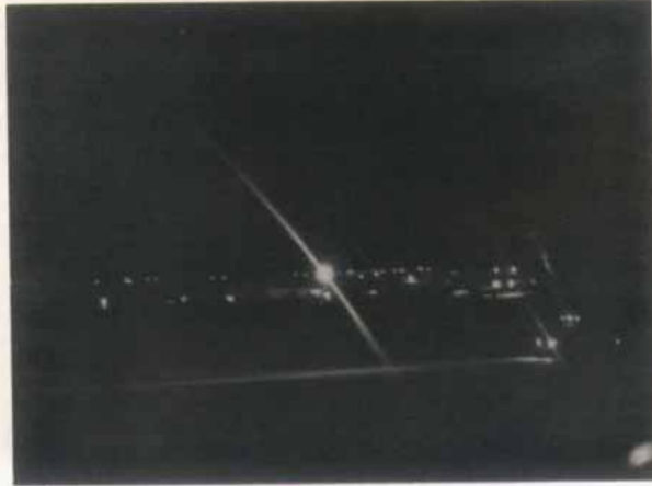
Figure 2.9: Diffraction of a point light source through a canopy.
