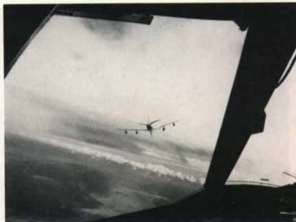
Figure 2.13: Distortion of an aircraft when viewed through the heater coating deletion line of a B-1B windscreen.
