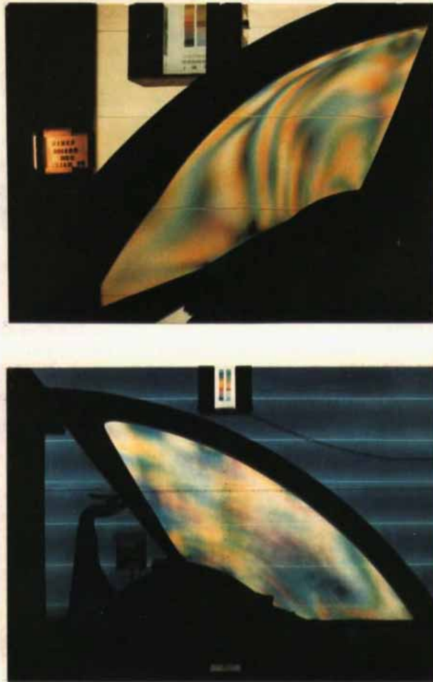
Figure 2.4: Birefringence patterns of F-111 windscreens produced by two different manufacturing techniques.
