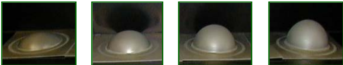
Figure 14 Bulge samples at various times during the forming process.
