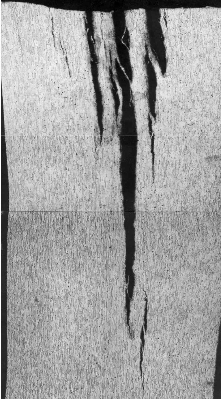
Figure 73. Optical Micrograph of Metallographic Cross Section Across the Secondary Crack Shown in Figures 71 and 72
