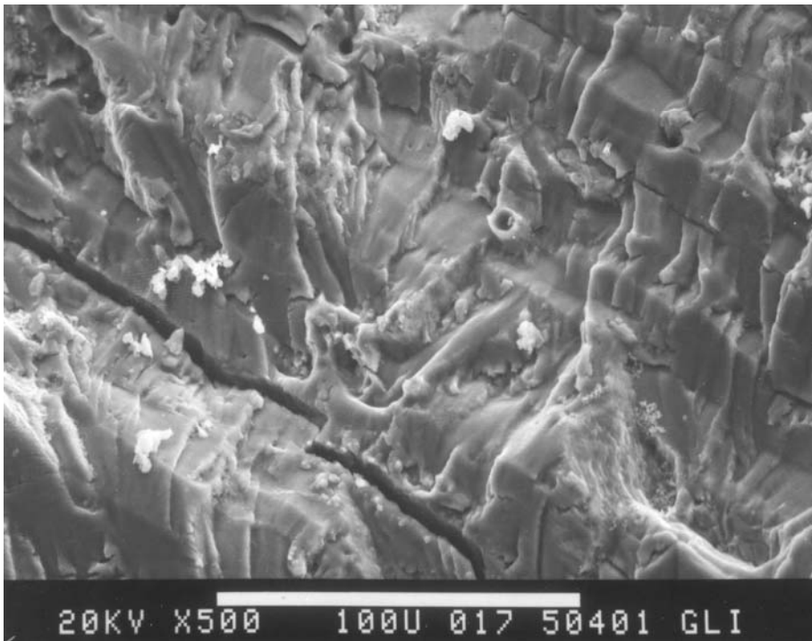
Figure 72. Detail of Secondary Crack Shown in Figure 71
