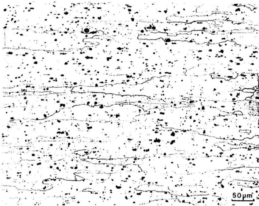
Figure 2. Optical Micrograph of Cross Section through Aluminum Alloy 2024-T3 Showing Elongated Grains and Constituent Particles
