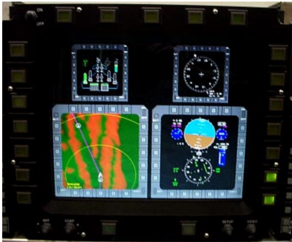
Figure 2. Cockpit simulator display (16.1 in.).
