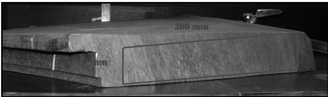
Figure 7. As Received As-Cast NAB Section of Prototype Hub (SideView)
