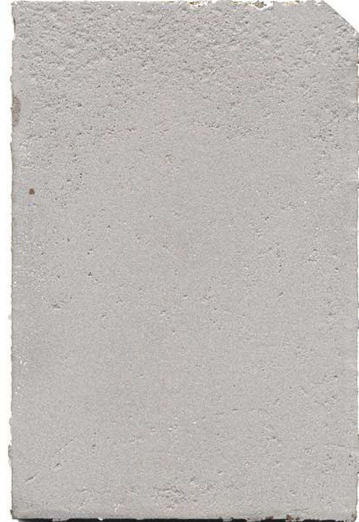
(b) Abrasive Blast + KLEENINHIB 486 + CHEMINHIB 420
