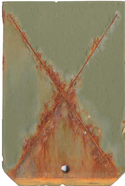
(c) Abrasive Blast + Spray Zinc Phosphate
