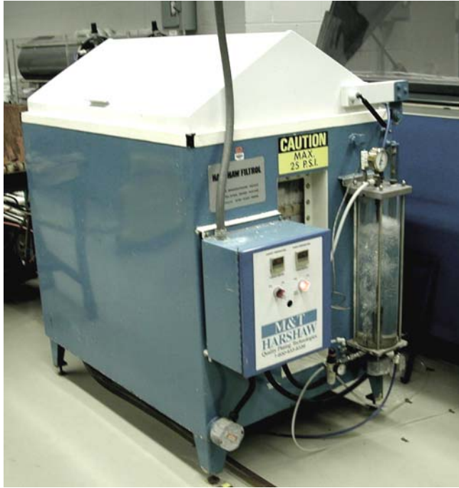
Figure 5. Test chamber configuration used for ASTM B 117-90 neutral salt fog.
