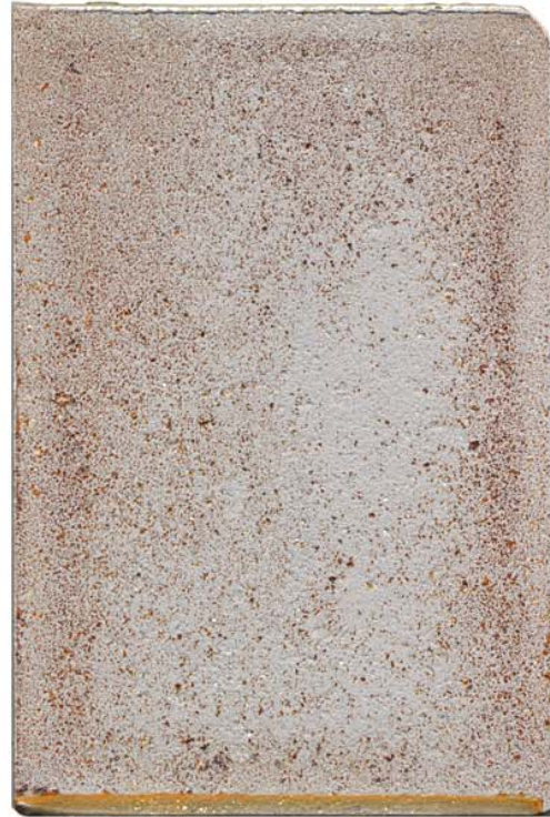
(b) Abrasive Blast + KLEENINHIB 486 + CHEMINHIB 420
