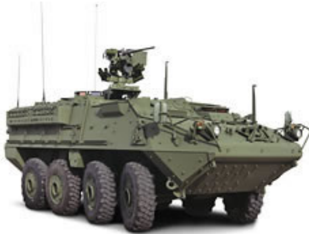
Figure 1. Brigade Combat Team (BCT) Stryker Interim Armored Vehicle (IAV) in Standard Infantry Carrier Vehicle (ICV) configuration.
