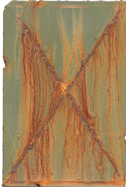
(b) Abrasive Blast + CHEMINHIB 420
