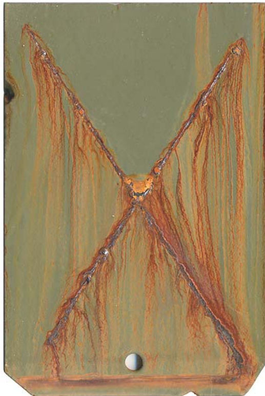
(c) Abrasive Blast + Spray Zinc Phosphate
