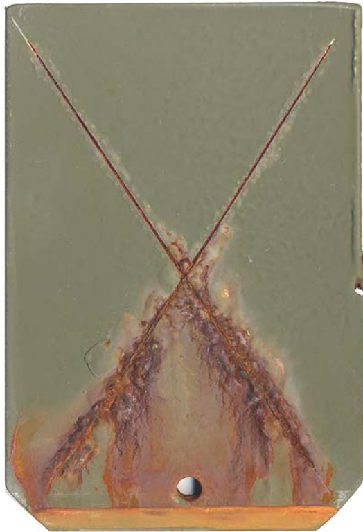
(c) Abrasive Blast + Spray Zinc Phosphate
