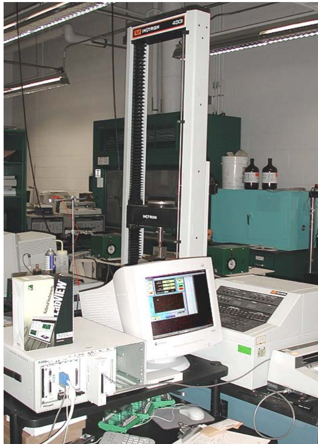
Figure 12. Rising step load test configuration.
