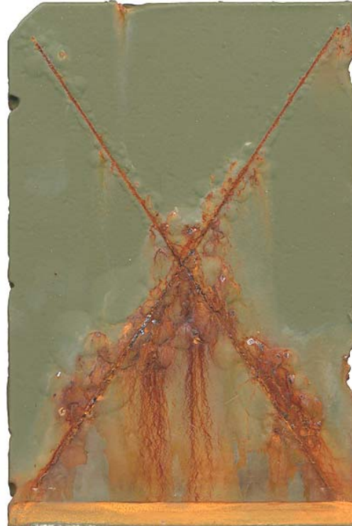
(b) Abrasive Blast + CHEMINHIB 420
