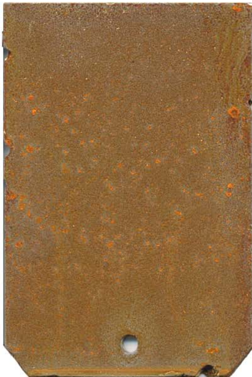
(c) Abrasive Blast + Spray Zinc Phosphate
