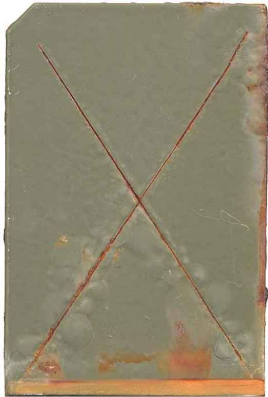
(b) Abrasive Blast + CHEMINHIB 420
