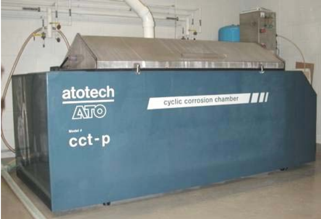
Figure 6. Test chamber configuration used for GM 9540P cyclic corrosion.
