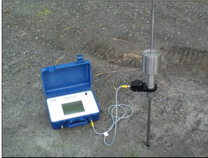
Figure 22. Dynamic cone penetrometer (DCP) for determining soil strength as a function of depth.
