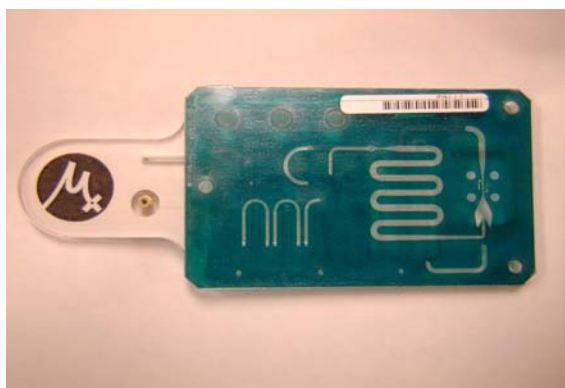
Figure 20. Three channel card showing lyse on the fly operation
