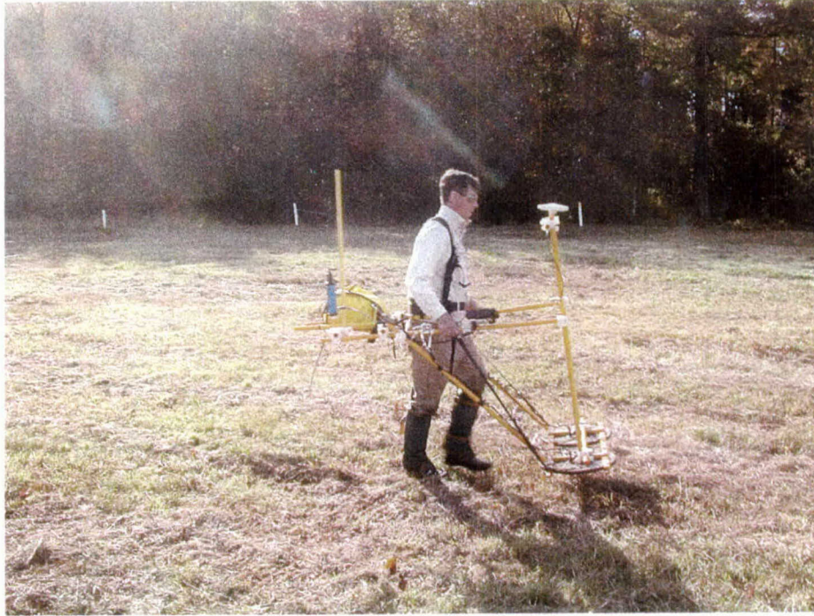
Figure 1. Dual sensor TM-5 EMU EM detector data acquisition system.
