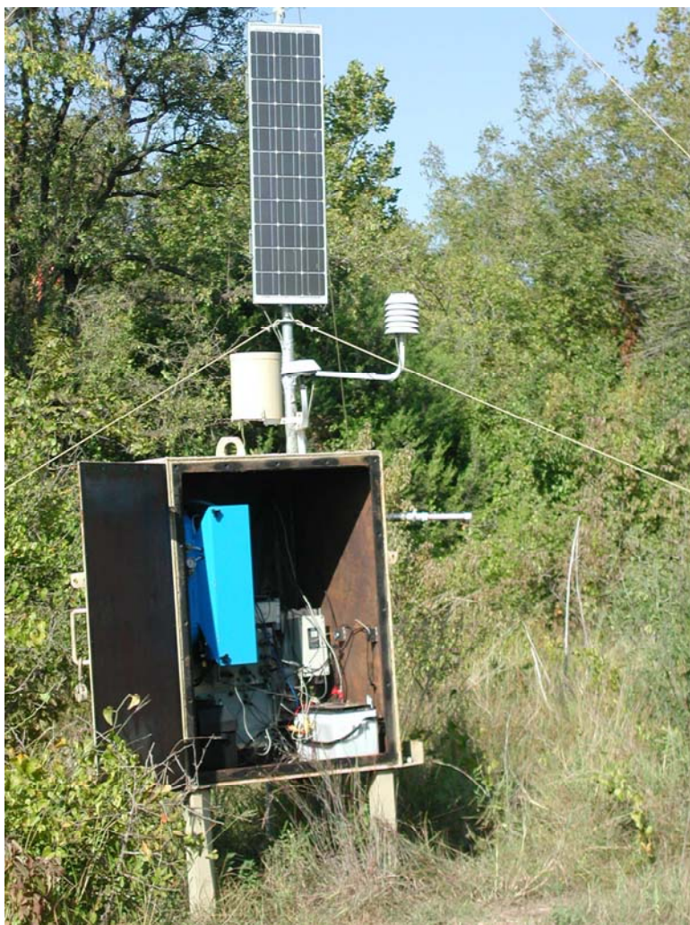
Figure 2. Enclosure and weather station instrumentation at House Creek.
