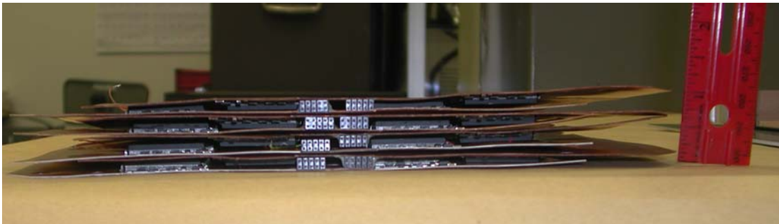
Figure 31: Eight nested frequency processor boards viewed end on
